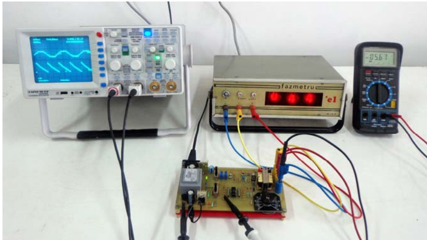
Fig.3.12 Image of the laboratory set-up by means of which it can be displayed the waveforms and it can be drawn the transfer function \alpha = f(V_{control}) of the UAA145.
