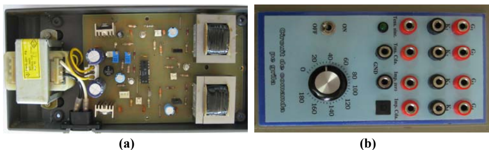
Fig. 3.11 Gate trigger circuit with UAA145 for different single-phase rectifiers (with maximum 4 thyristors – see Fig.3.5) ; (a) inside case picture; (b) front case picture.
