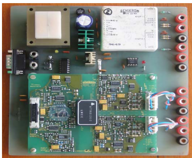
Fig 6.11 The image of the control circuit achieved with SKHI hybrid dual drivers.
