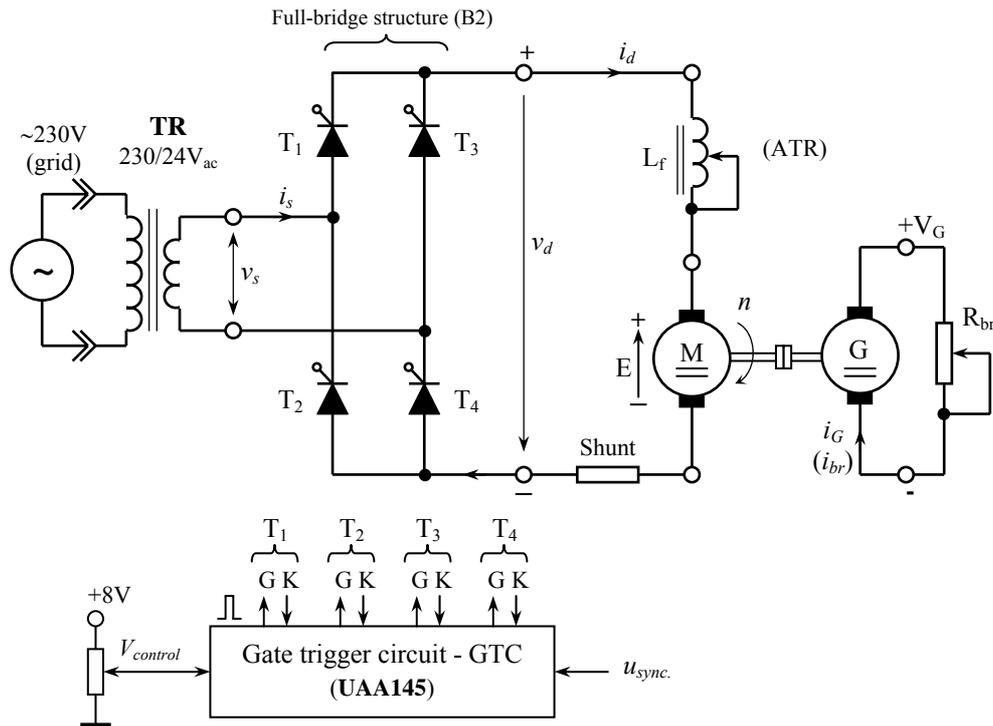
**Fig. 8.12** Block diagram of the laboratory setup – single-phase bridge rectifier (B2) with an  $R-L-E$  active load.
