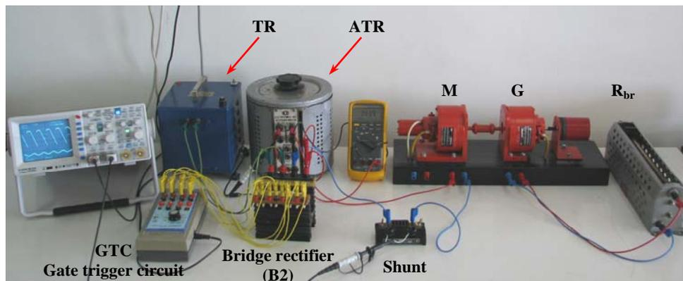
**Fig. 8.13** Image of the laboratory application.
