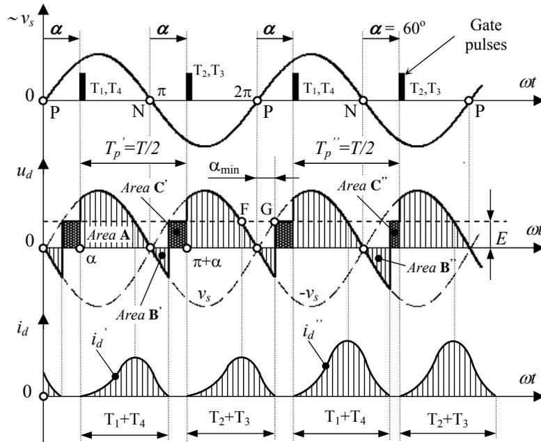
**Fig. 8.11** Discontinuous conduction mode in the case of a single-phase rectifier with a  $R-L-E$  load ( $\alpha=60^\circ$  [el]).
