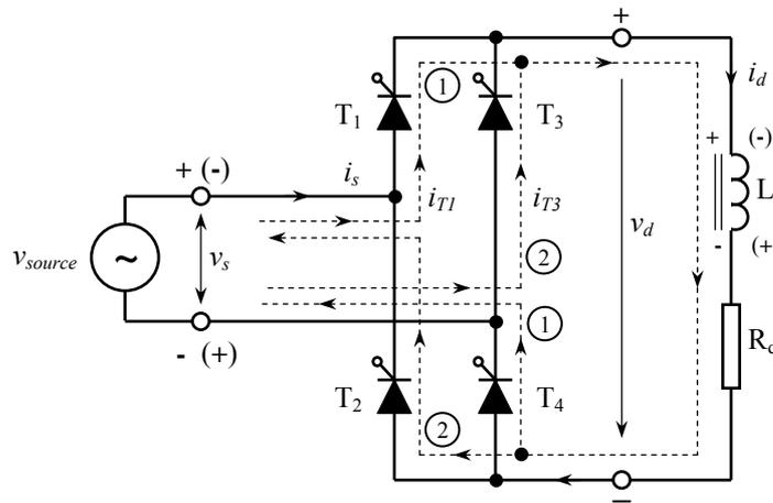
**Fig. 8.8** Phase-controlled rectifier with resistive-inductive load.
