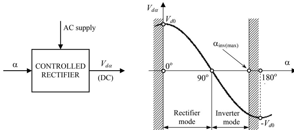
**Fig. 8.4** Adjustment characteristic of a phase-controlled rectifier:  $V_{d\alpha} = f(\alpha) = V_{d0} \cdot \cos \alpha$ .
