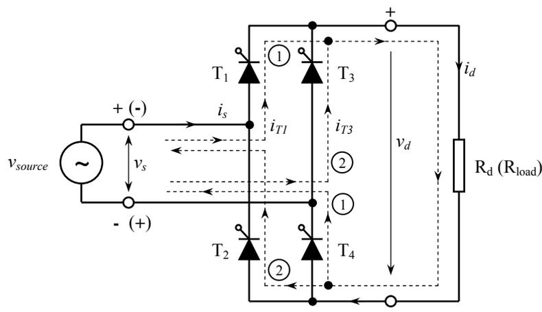
Fig. 8.5 Phase-controlled rectifier with a purely resistive load.
