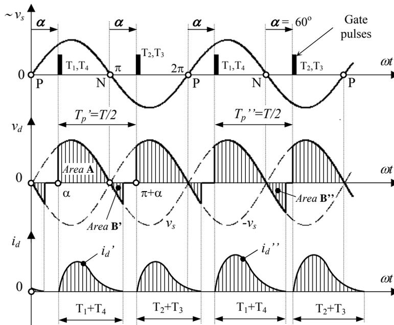
**Fig.8.9** Discontinuous conduction mode in the case of a single-phase rectifier with a resistive-inductive load ( $\alpha=60^\circ$  [el]).
