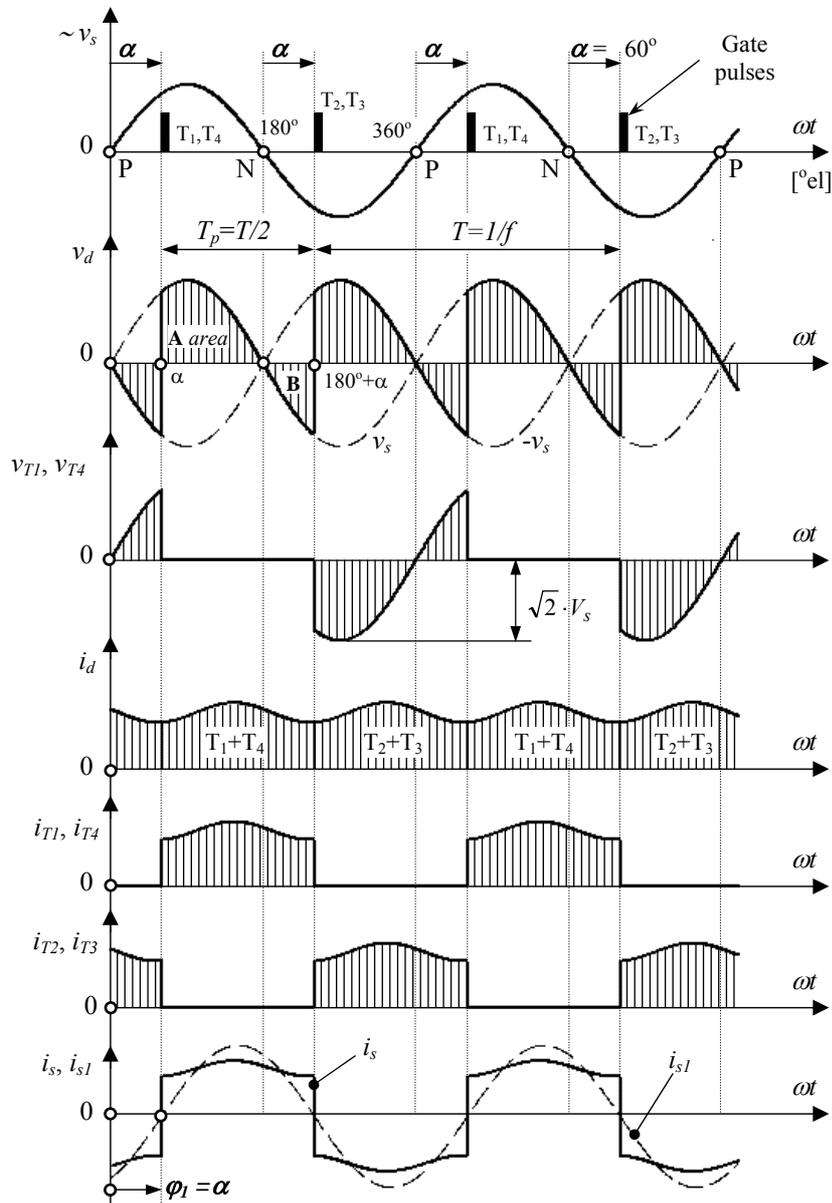
**Fig. 8.3** Waveforms corresponding to a single-phase bridge rectifier with thyristors controlled with the firing angle  $\alpha=60^\circ$  [el].
