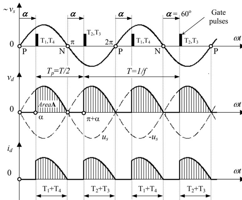
**Fig. 8.6** Discontinuous conduction mode waveforms for a single-phase rectifier with a purely resistive load ( $\alpha=60^\circ$  [el]).
