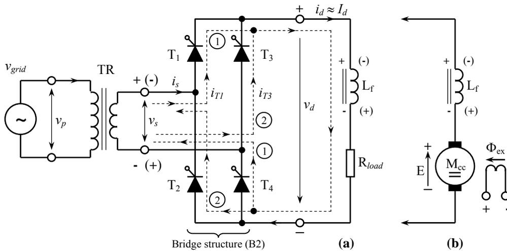
**Fig. 8.1** Single-phase full-bridge rectifier with: (a) R-L load; (b) R-L-E load.
