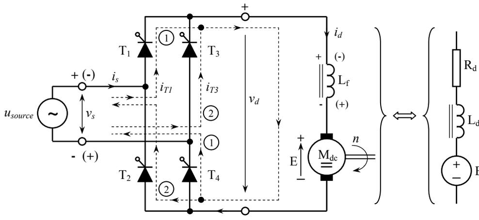
**Fig.8.10** Phase-controlled rectifier with R-L-E load.
