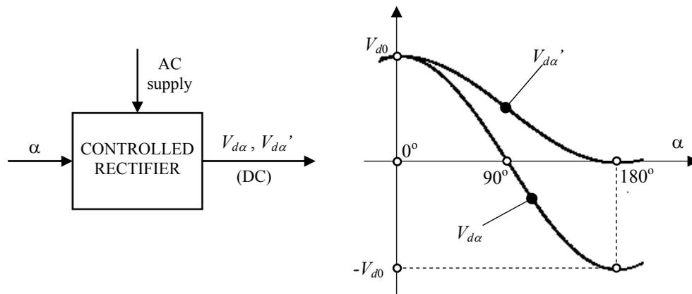
**Fig. 8.7**  $V_{d\alpha} = f(\alpha)$  for a rectifier with filter inductance and continuous conduction mode;
