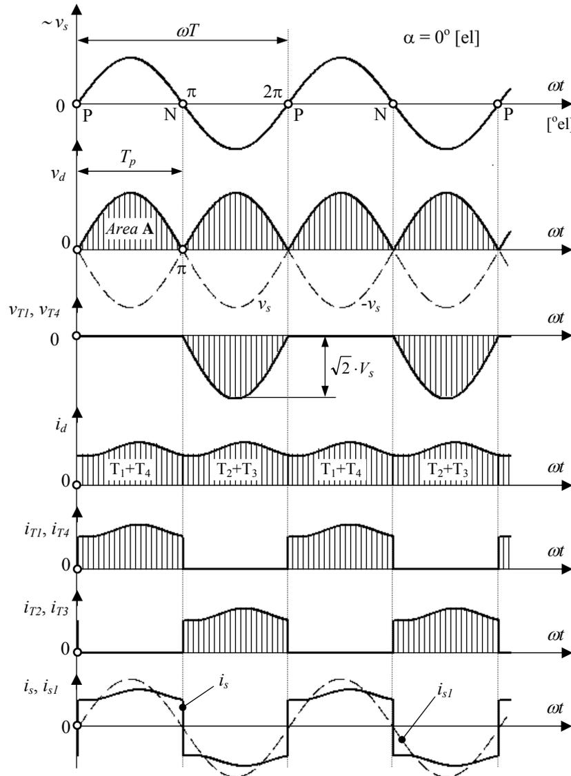
**Fig. 8.2** The waveforms of a single-phase bridge rectifier achieved with diodes or with thyristors controlled with the firing angle  $\alpha=0^\circ$  (continuous conduction mode).
