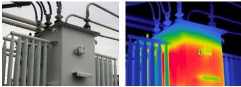
Figure 2. – Electrical transformer thermal imaging
