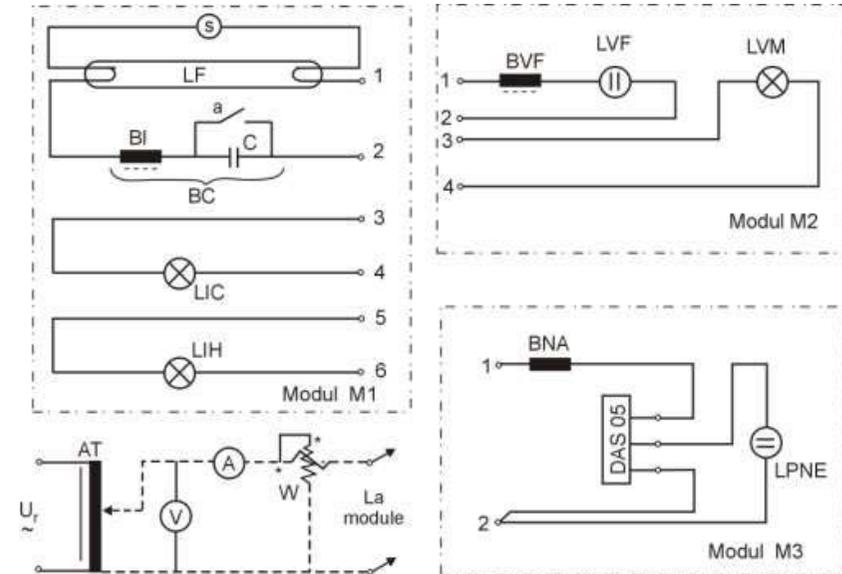
Fig.2.11. Assembly for the determination of transitory regime parameters and the operating one of the light source.
